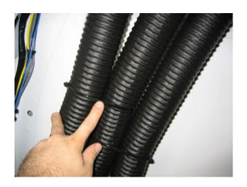
When routing the hoses, tie together using 15" wire ties, to keep a neat and tight fit to the wall of the vehicle.
